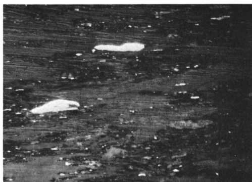
Figure 1. Thin section of a coal. The majority of the sample is vitrinite; light spots are sphoronite and dark spots are attrital (courtesy of W. C. Grady Coal Research Bureau, West Virginia University).
